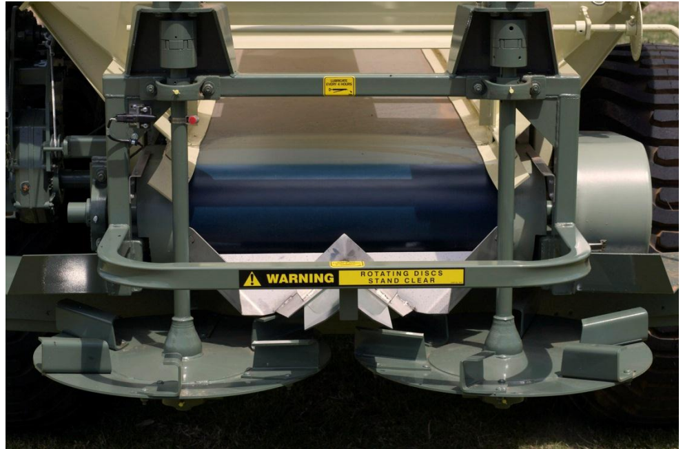
Type C Spinner System introduced in 2007
