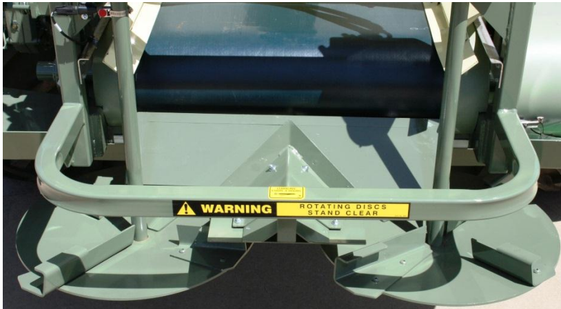
The new Type D Spinner, Vane and Chute Configuration For more information see MMS-SPN-MKT-001_Type D Spinners Info sheet
