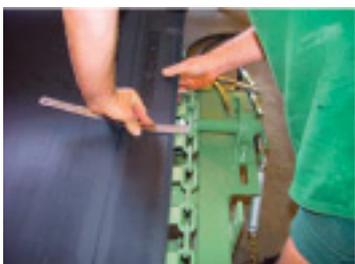
4. Clamp the feedchain to the joiner slat.
