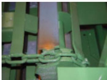
2. Position the rubber supplied so that one end is flush with the back edge of the joiner slat.
